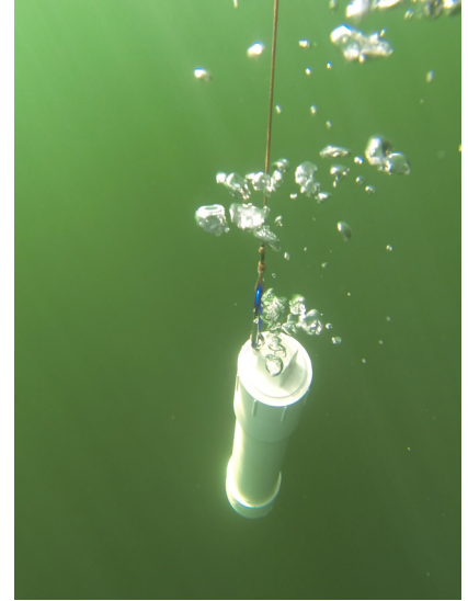
A composite sampler used to collect chlorophyll-a samples
